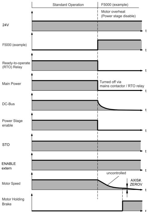
If the drive detects the motor to be at zero velocity (AXIS#.ZEROV) or timeout occurs (AXIS#.ZEROT), the motor brake is applied ( $\rightarrow$  # 109). Set parameter AXIS#.MOTOR. BRAKEIMM to 1 with vertical axes, to apply the motor holding brake immediately after faults.
