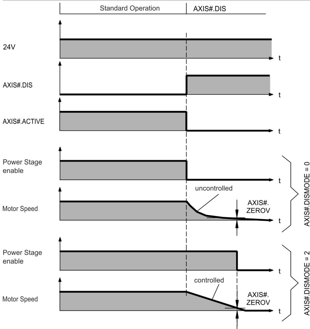
If the drive detects the motor to be at zero velocity (`AXIS#.ZEROV`) or timeout occurs (`AXIS#.ZEROT`), the motor brake is applied (→ # 109).
