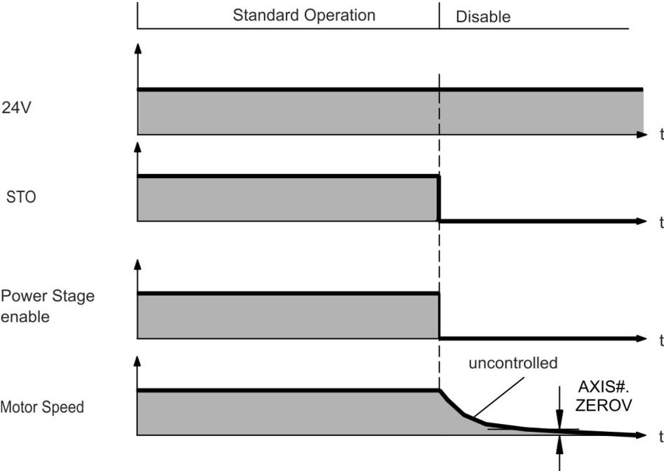
If the drive detects the motor to be at zero velocity (AXIS#.ZEROV) or timeout occurs (AXIS#.ZEROT), the motor brake is applied (→ # 109). Set parameter AXIS#.MOTOR. BRAKEIMM to 1 with vertical axes, to apply the motor holding brake immediately after STO.
