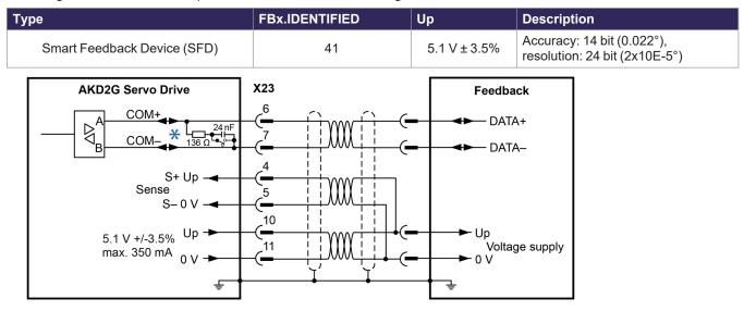
\*SFD must always use AC coupled termination - DC termination switch open.
