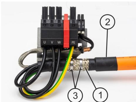
1. Strip the external cable sheath to a length of approx. 80mm, taking care not to damage the braided shield.
