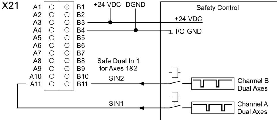
Dual channel for axis1 and axis2, Emergency Stop, automatic restart (example for default configuration):
