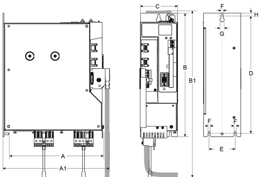
**NOTE** Outline width and height dimensions are measured on footprint level (mounting plate). Dimensions on the front plate are slightly smaller.
