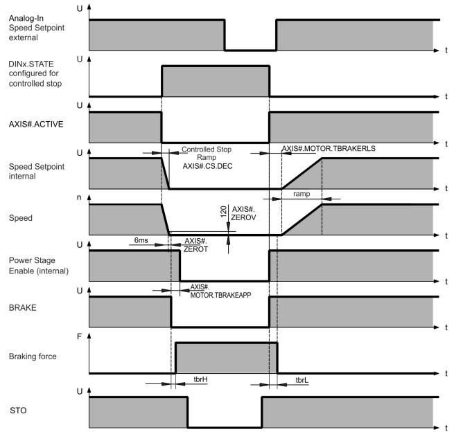
The drive speed setpoint is internally driven down an adjustable ramp (AXIS#.CS.DEC) to 0 V.
