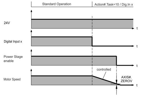
If the drive detects the motor to be at zero velocity (AXIS#.ZEROV) or timeout occurs (AXIS#.ZEROT), the motor brake is applied ( $\rightarrow$  # 109).
