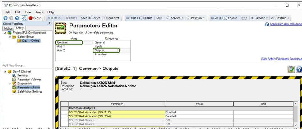
If the application requires dual channel outputs for a status message, enable the output pair to be used.
