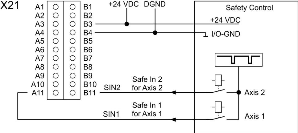
Single channel for axis1 and axis2, Emergency Stop, automatic restart:
