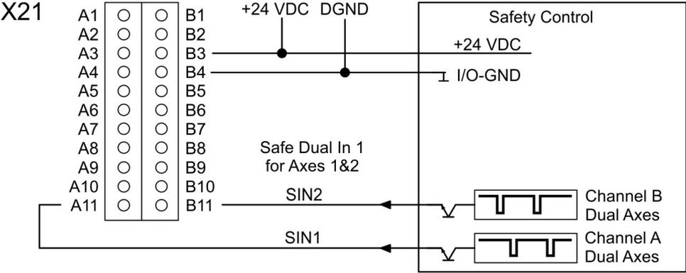
Dual channel for axis1 and axis2, Safety Control with relay contacts, automatic restart:
