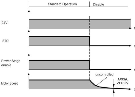
If the drive detects the motor to be at zero velocity (AXIS#.ZEROV) or timeout occurs (AXIS#.ZEROT), the motor brake is applied ( $\rightarrow$  # 109). Set parameter AXIS#.MOTOR. BRAKEIMM to 1 with vertical axes, to apply the motor holding brake immediately after STO.
