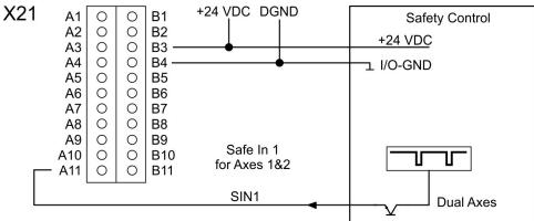
Single channel, 2 axes, Safety Control with relay contacts, automatic restart (distinct pulse monitoring must be disabled):
