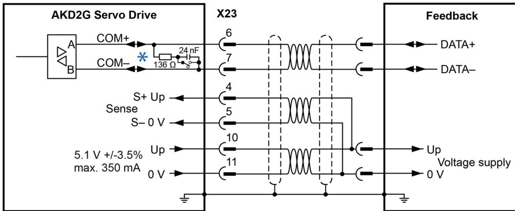
\* SFD must always use AC coupled termination - DC termination switch open.
