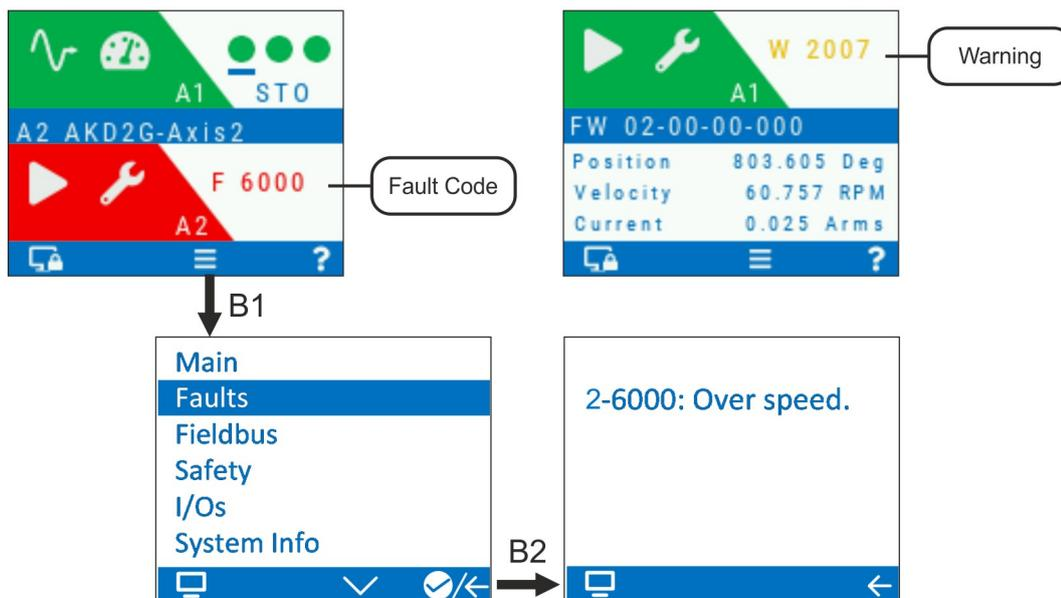
You can retrieve faults on a per-axis basis with the parameter: `AXIS#.FAULTS`, where # is the Axis number. For retrieving warnings use `AXIS#.WARNINGS`, or `DRV.WARNINGS`.
