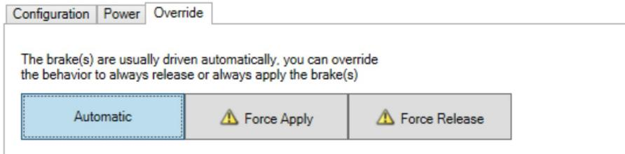
Manual control of the brakes is prohibited when SBC muting is not active and STO/SBC is active at the same time.
