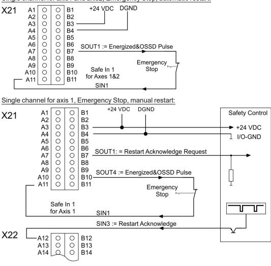
Single channel for axis1 and axis2, Emergency Stop, automatic restart:
