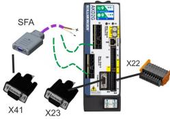
AKD2G offers up to 5 feedback channels, which may be used as the command source for electronic gearing or EEO (Emulated Encoder Output) or Master-Slave.
