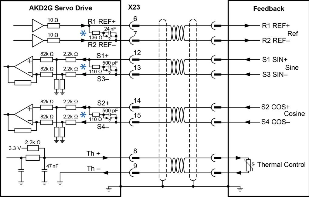
\* Resolver Sine/Cosine channels must be high impedance - DC termination switch open.
