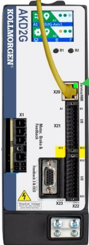
Confirm that the link LEDs on the drive (green LED on the RJ45 connector) and on your PC are both illuminated. If both LEDs are illuminated, then you have a working electrical connection. The LCD display shows a sign, if the connection between AKD2G and WorkBench is active.
