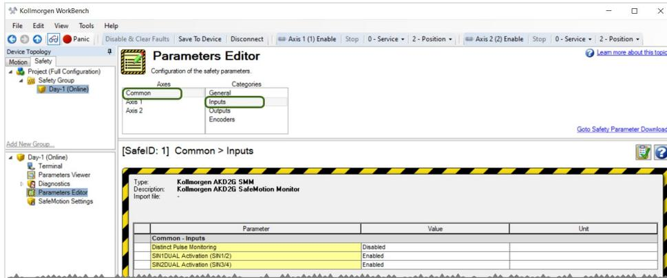
Define the required monitoring for OSSD test pulses (→ # 213). If the application requires dual channel inputs for a safety function, enable the safe input pair to be used.
