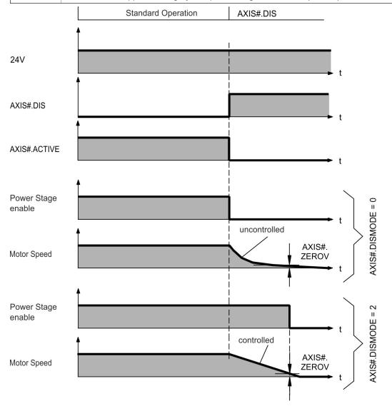
If the drive detects the motor to be at zero velocity (AXIS#.ZEROV) or timeout occurs (AXIS#.ZEROT), the motor brake is applied ( $\rightarrow$  # 109).
