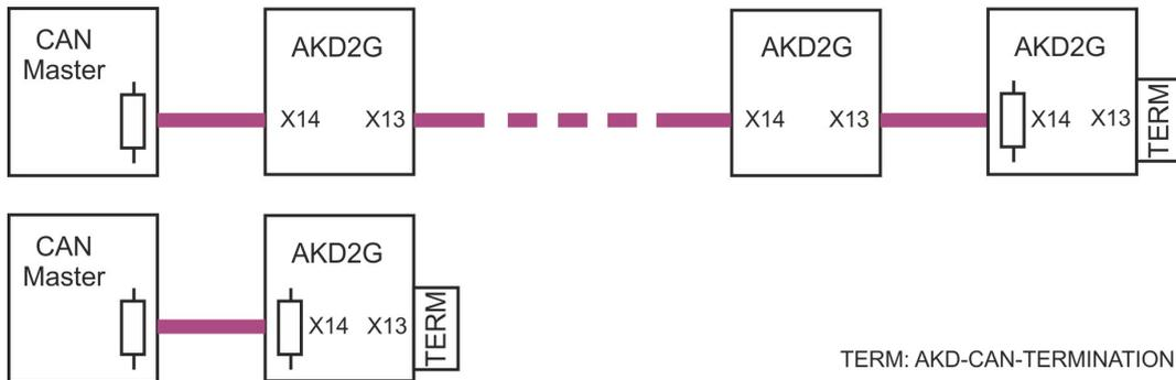
**NOTE** Remove the termination connector if the AKD2G is not the last CAN-Bus device and use X13 for connecting the next CAN node.
