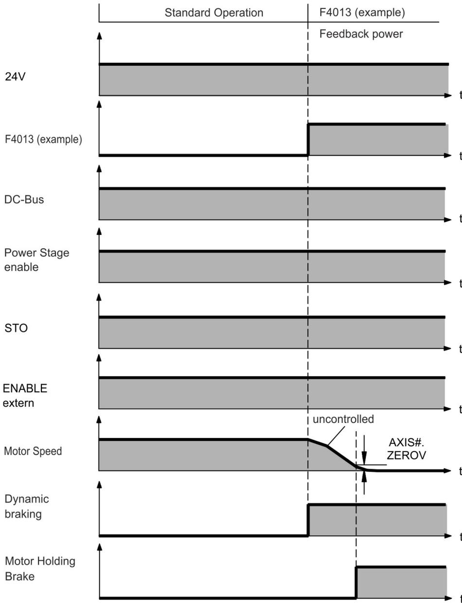
If the drive detects the motor to be at zero velocity (AXIS#.ZEROV) or timeout occurs (AXIS#.ZEROT), the motor brake is applied (→ # 109).
