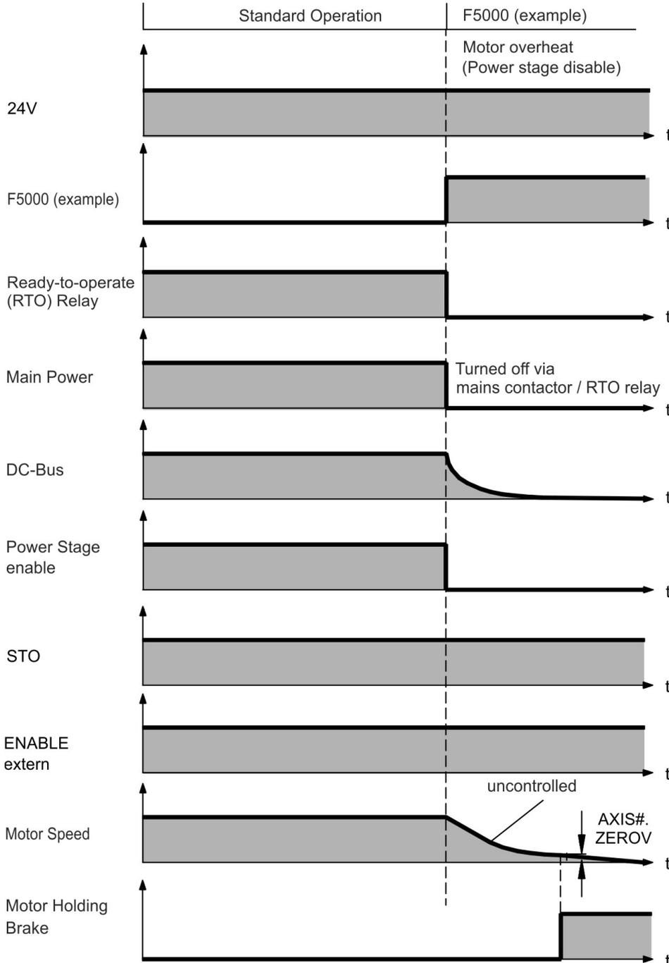
If the drive detects the motor to be at zero velocity (AXIS#.ZEROV) or timeout occurs (AXIS#.ZEROT), the motor brake is applied (→ # 109). Set parameter AXIS#.MOTOR.BRAKEIMM to 1 with vertical axes, to apply the motor holding brake immediately after faults.
