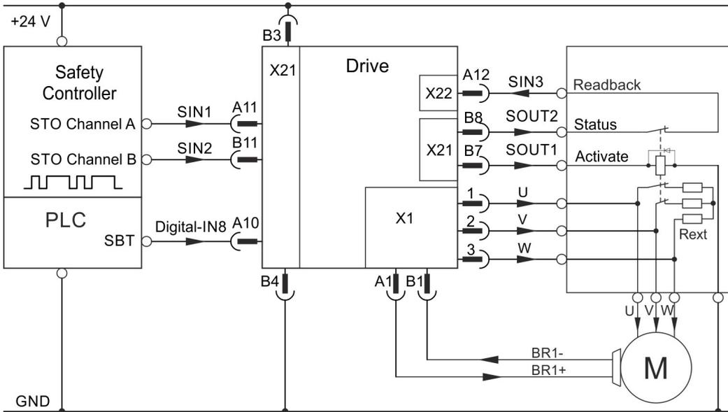
**Example: STO activated by safe inputs, SDB dual channel, SIL3 PLe, SBC, SBT**
