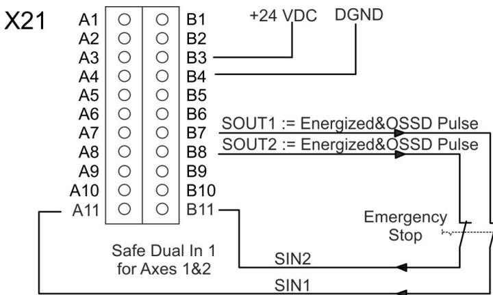
Dual channel for axis1 and axis2, Emergency Stop, manual restart:
