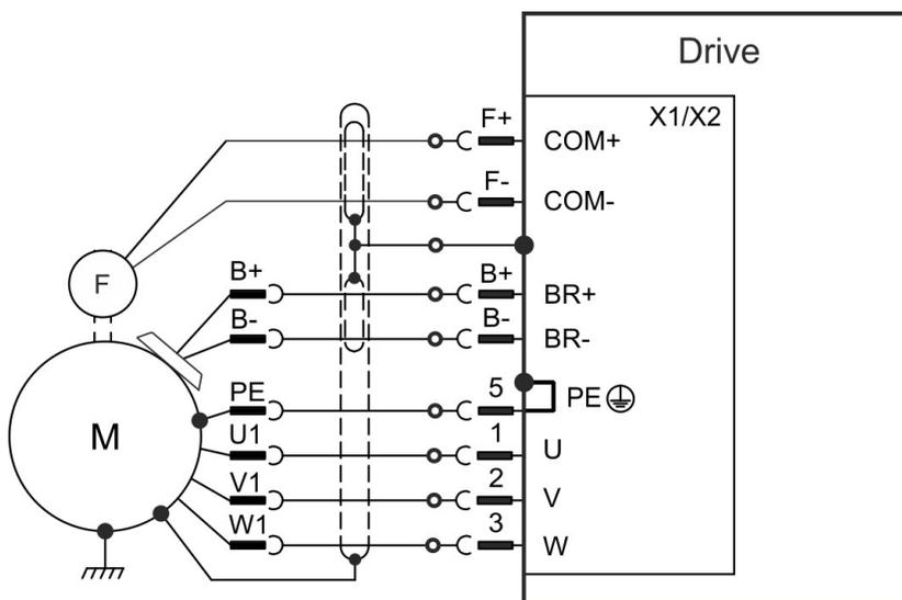
Pinout is identical for connectors X1 and X2.
