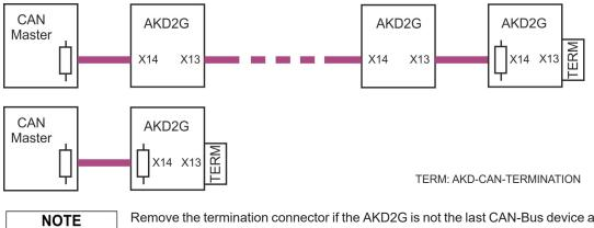
Remove the termination connector if the AKD2G is not the last CAN-Bus device and use X13 for connecting the next CAN node.
