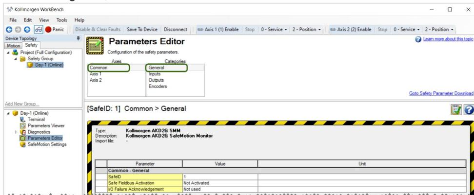
The SafeID (set with the rotary switches on the drive) is visible in the first line.
