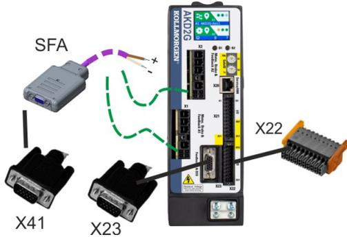
AKD2G offers up to 5 feedback channels, which may be used as the command source for electronic gearing or EEO (Emulated Encoder Output) or Master-Slave.
