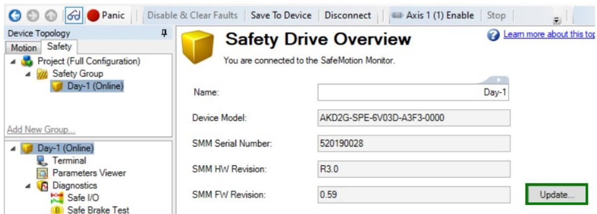
3. The **Safety Firmware Update** view will appear. Select the drive(s) and fill in the required information: the update password, firmware checksum, and firmware file.
