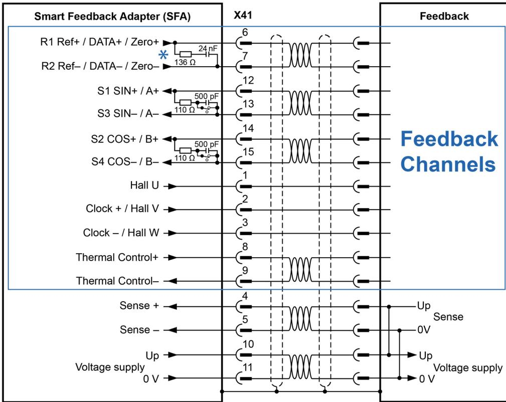
\* The SFA does not include a DC termination switch across pins 6 and 7.
