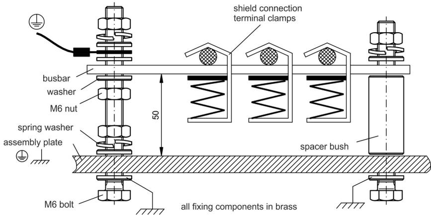
2. Squeeze together the coil spring and the supporting plate and push the busbar through the opening in the holder.
