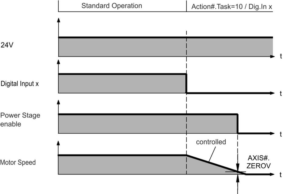
If the drive detects the motor to be at zero velocity (AXIS#.ZEROV) or timeout occurs (AXIS#.ZEROT), the motor brake is applied (→ # 109).
