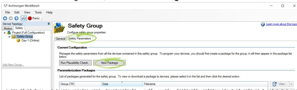
The new package is then listed underneath the Parameterization Packages section.
