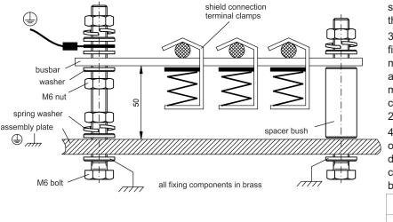
2. Squeeze together the coil spring and the supporting plate and push the busbar through the opening in the holder.
