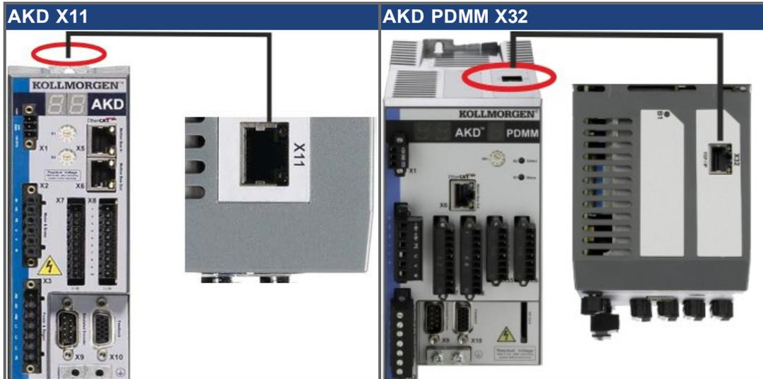
Connect the service interface (X11 or X32) of the drive to an Ethernet interface on the PC directly or via a network hub/switch, **while the supply to the equipment is switched off**. Use standard Cat. 5 Ethernet cables for connection (in some cases crossover cables will also work).
