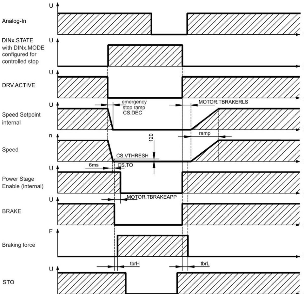
The speed setpoint of the drive is internally driven down an adjustable ramp (CS.DEC) to 0 V. With default values the output for the brake is switched on when the speed has reached 120 rpm (CS.VTHRESH) for at least 6 ms (CS.TO). The rise ( $t_{brH}$ ) and fall ( $t_{brL}$ ) times of the holding brake that is built into the motor are different for the various types of motor (see motor manual).
