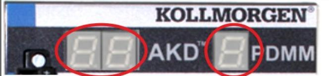
A photograph of a Kollmorgen AKD-M drive's LED display. The display shows two digits, both of which are '8', followed by a single digit which is '8'. The text 'KOLLMORGEN®' is visible above the display, and 'AKD™' and 'PDMM' are visible to the right. Red circles highlight the two-digit and one-digit displays.                  |
