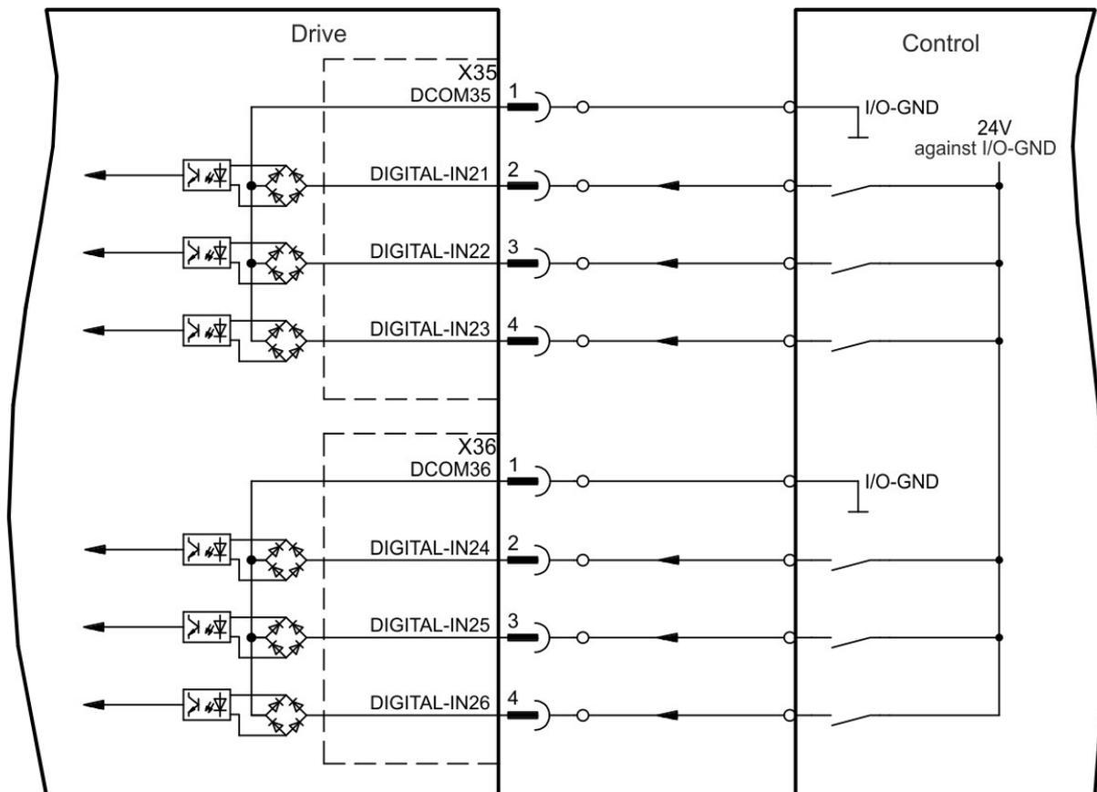
Digital Input Wiring Diagram (Sink type connection, example)
