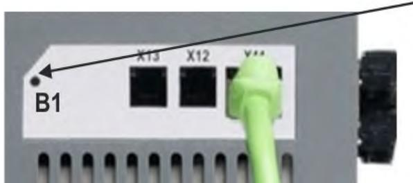
3. When the display blinks with the set rotary switch setting stop pushing B1 and wait until the blinking stops. During that time the parameter FBUS.PARAM01 is set to the new value and all parameters are stored to the non volatile memory. The new setting will be taken with the next power-up of the drive.
