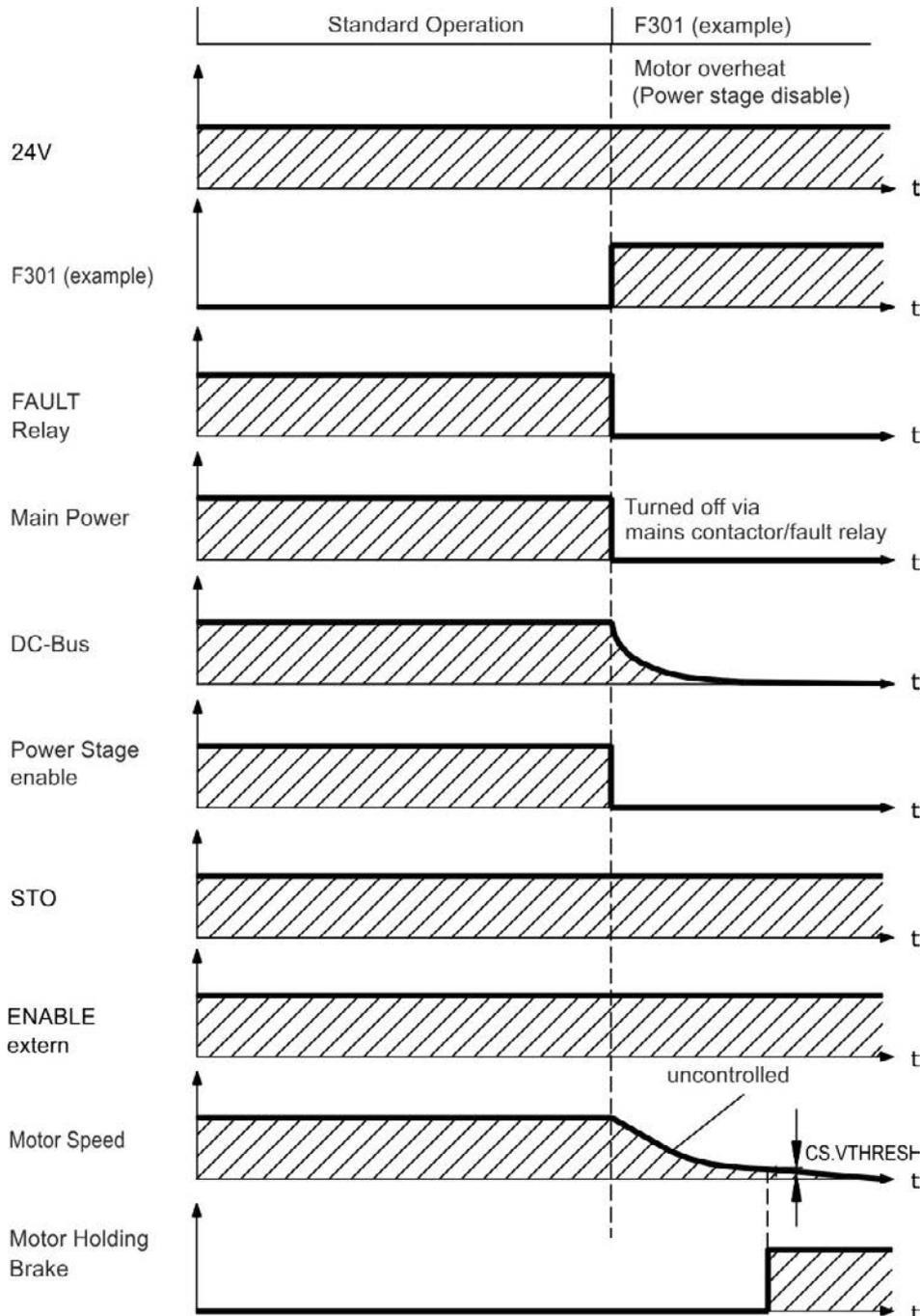
If velocity drops below threshold  $CS.VTHRESH$  or timeout occurs the motor holding brake is applied (=> p. 98). Set parameter `MOTOR.BRAKEIMM` to 1 with vertical axes, to apply the motor holding brake immediately after faults.
