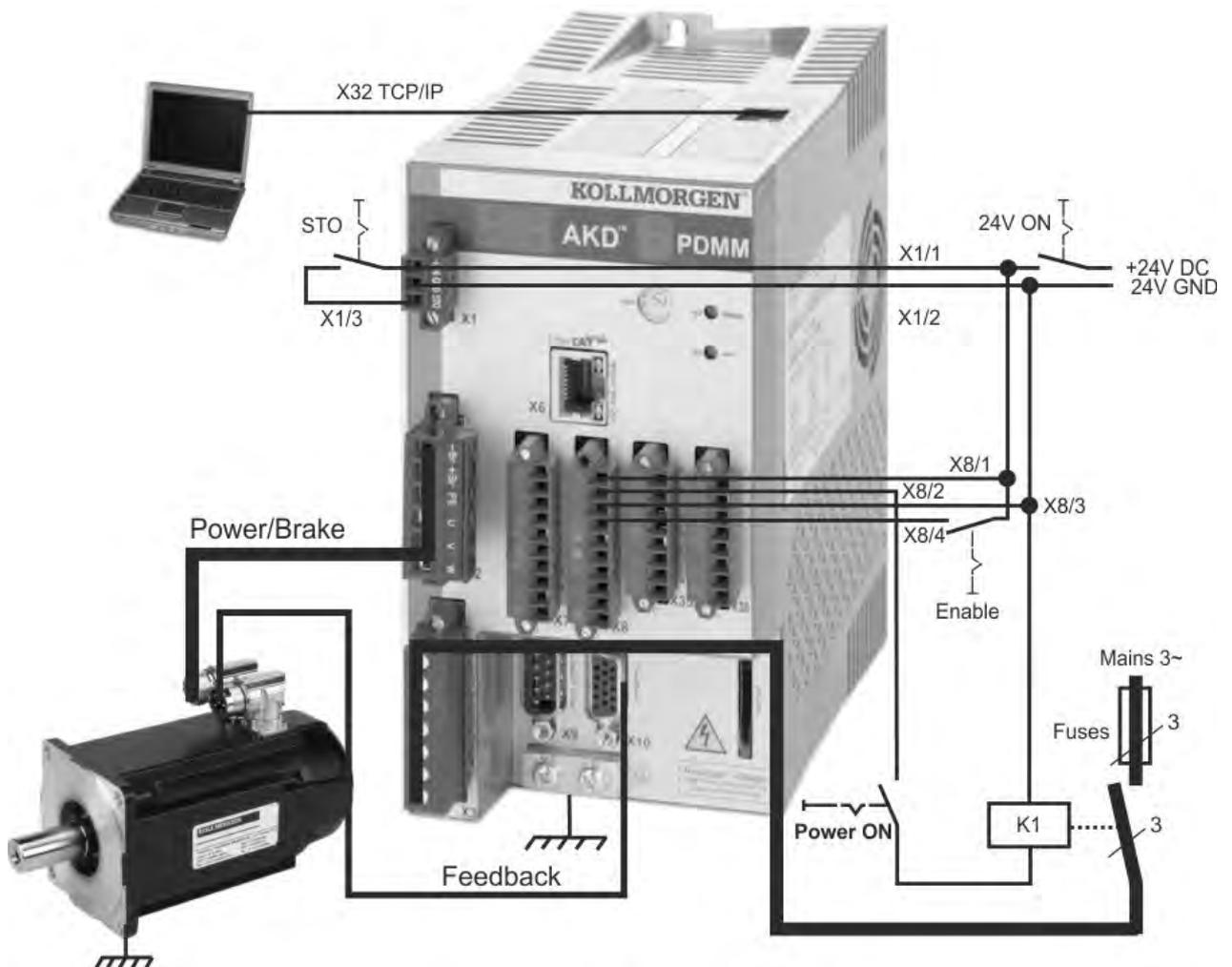
When connecting the AKD PDMM directly to a PC, static IP addressing (not 0) is recommended.
