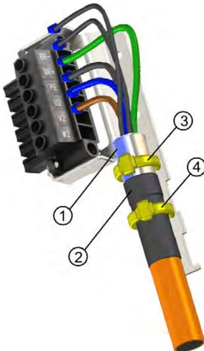
Strip the external cable sheath to a length of approx. 120 mm, taking care not to damage the braided shield. Push the braided shield (1) back over the cable and secure with a rubber sleeve (2) or shrink sleeve.
