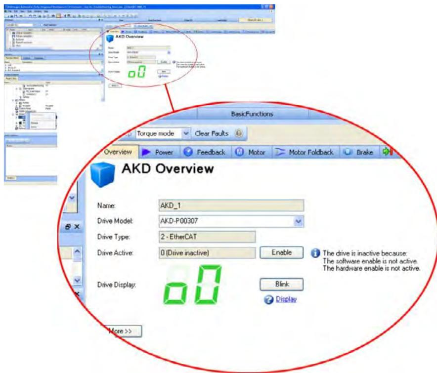
Additionally the setup wizard will take you through a set of steps to perform the configuration:
