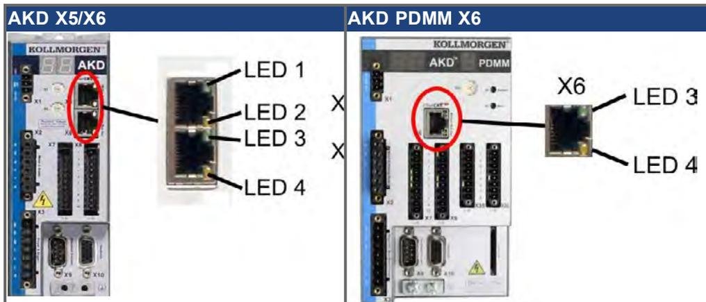
**NOTICE** Do not connect the Ethernet line for the PC or PAC with the set up software to the motion bus interface X5/X6. The set up Ethernet cable must be connected to X11 or X32.
