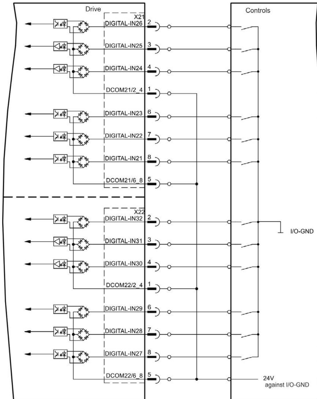
Digital Input Wiring Diagram (Sink type connection, example)
