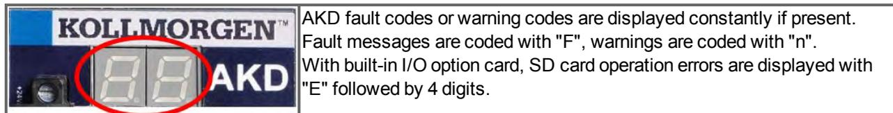
The left side of the LED displays F (or E) for a fault or n for a warning. The right side displays the fault or warning number as follows: 1-0-1-[break]. The highest priority fault is displayed. Multiple faults may be present when a fault condition is occurring. Check the AKD WorkBench Fault Screen or read the status of DRV.FAULTS through the controller or HMI for the entire list of faults.
