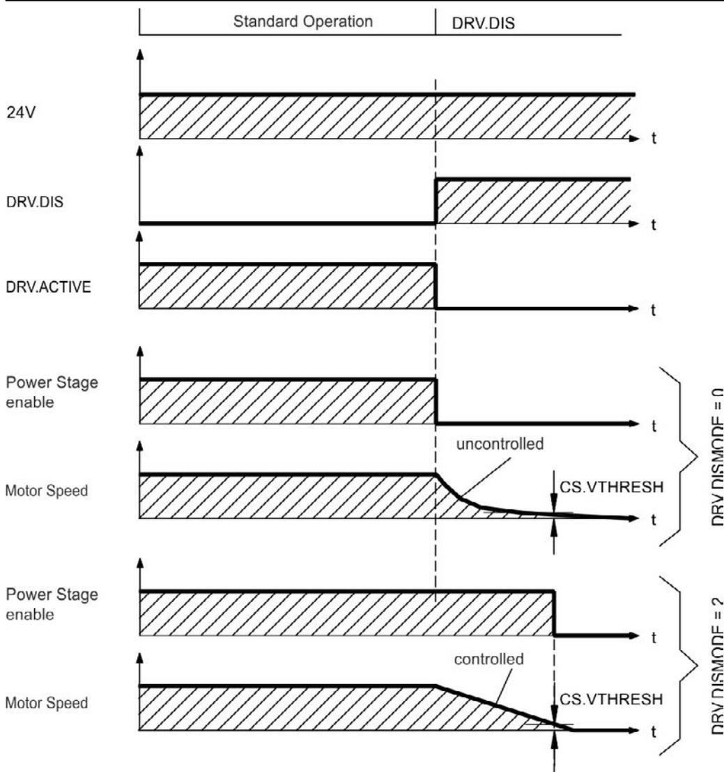
If velocity drops below threshold *CS.VTHRESH* or timeout occurs brake is applied (=> p. 98).
