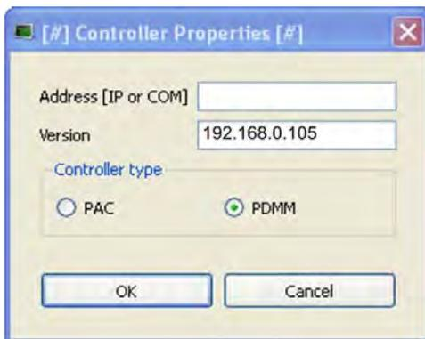
Type in the IP address of the AKD PDMM, set the **Controller Type** to PDMM and click OK. To connect to the PDMM, download, and run the project use the following controls:
