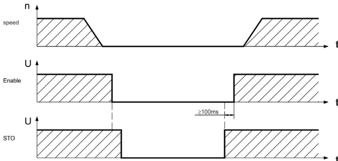
**⚠ WARNING** Suspended loads can set themselves in motion on motors without a brake, because the motor loses all torque when STO function is engaged (STO open and/or 0 V). Use motors with a built-in holding brake.
