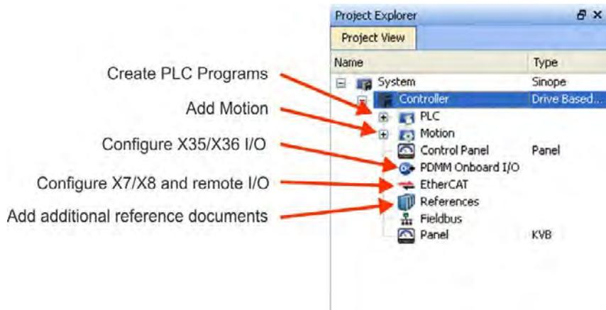
All drives, including the drive in the AKD PDMM itself, and the Remote I/O can be configured by the KAS IDE. Add the drives to the project: click on the EtherCAT item and scan for devices (1).
