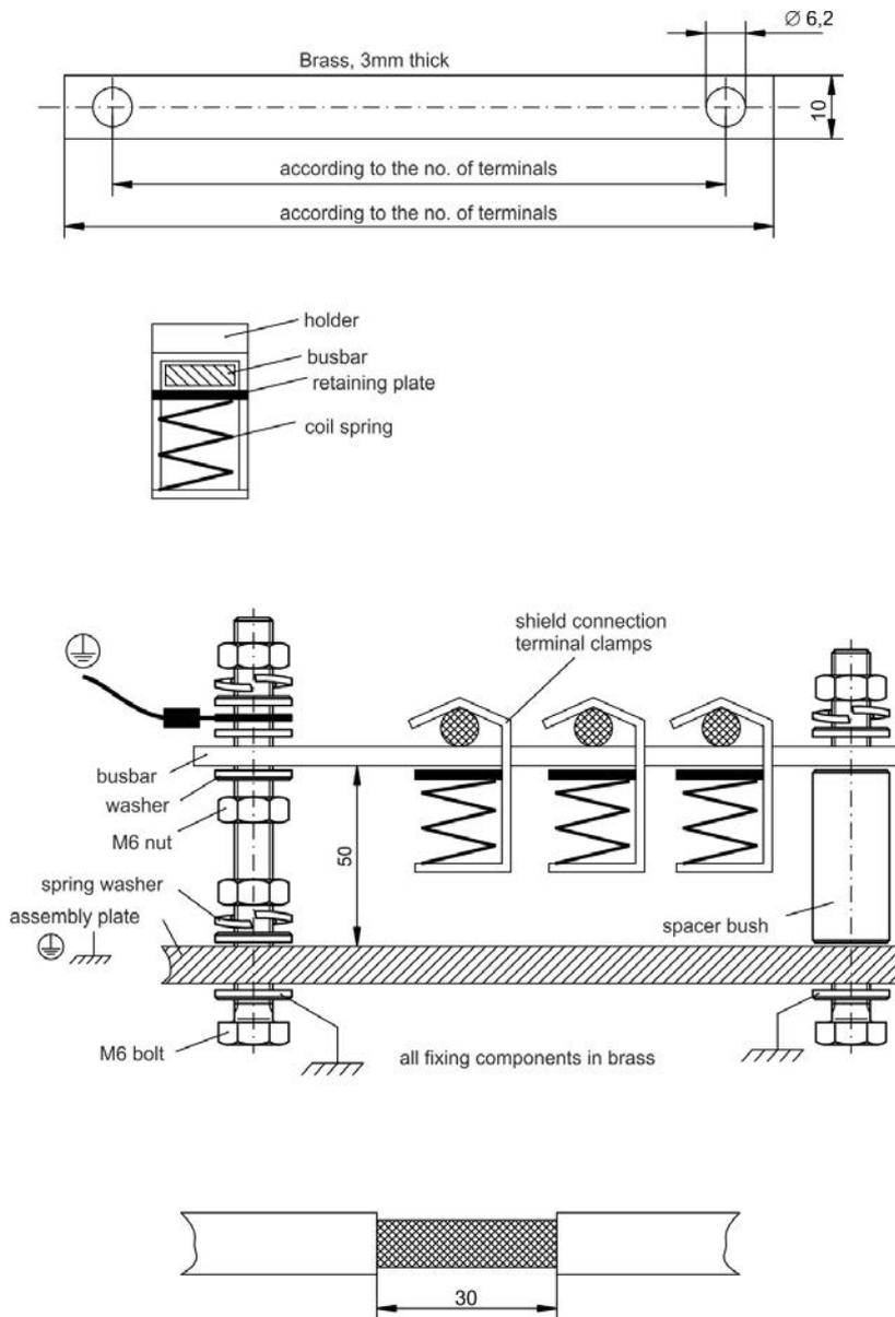
1. Cut a busbar of the required length from a brass rail (cross-section 10 x 3 mm) and drill holes in it as indicated. All shield clamps required must fit between the drill holes.
