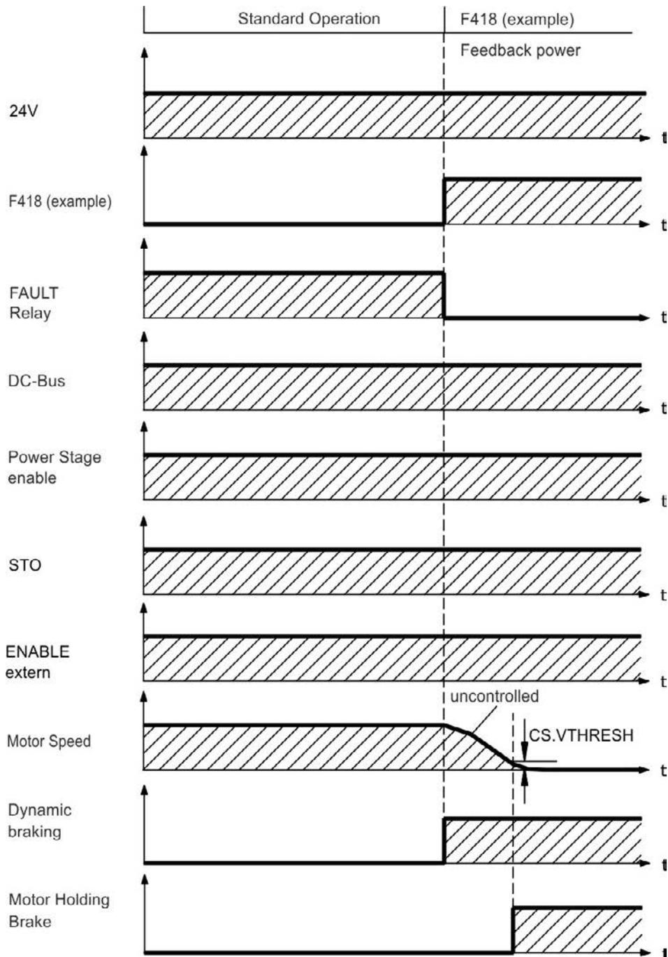
If velocity drops below threshold  $CS.VTHRESH$  or timeout occurs brake is applied (=> p. 98).
