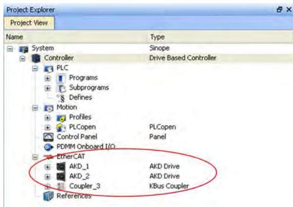
To communicate directly with a drive without running a project click on the EtherCAT item in the project tree. Click on the drive in the project tree to configure (1), then click on the **Online Configuration** button (2):
