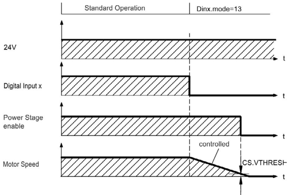
If velocity drops below threshold  $CS.VTHRESH$  or timeout occurs brake is applied (=> p. 98).
