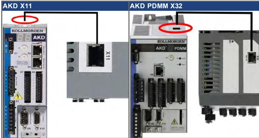
Connect the service interface (X11 or X32) of the drive to an Ethernet interface on the PC directly or via a network hub/switch, **while the supply to the equipment is switched off**. Use standard Cat. 5 Ethernet cables for connection (in some cases crossover cables will also work).
