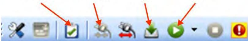
Double click on EtherCAT in the project view to open the EtherCAT devices view. Click on scan devices in the upper-right corner, and the KAS IDE will automatically identify and add your drive.
