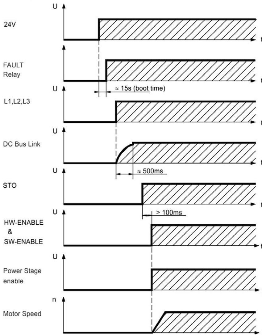
Fault F602 occurs when STO ( $\Rightarrow$  p. 53) does not have current when HW enable becomes active.
