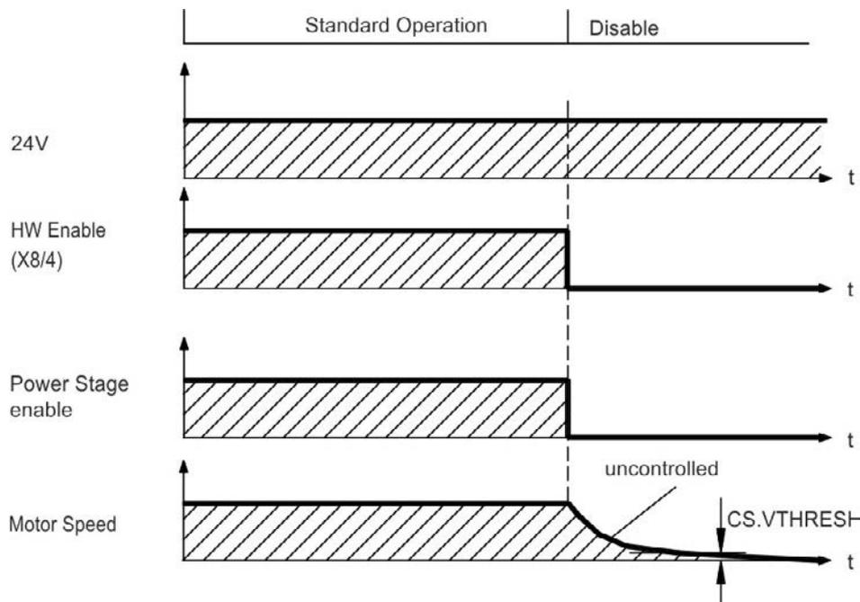
If velocity drops below threshold  $CS.VTHRESH$  or timeout occurs the motor holding brake is applied (=> p. 98). Set parameter  $MOTOR.BRAKEIMM$  to 1 with vertical axes, to apply the motor holding brake immediately after Hardware Disable.
