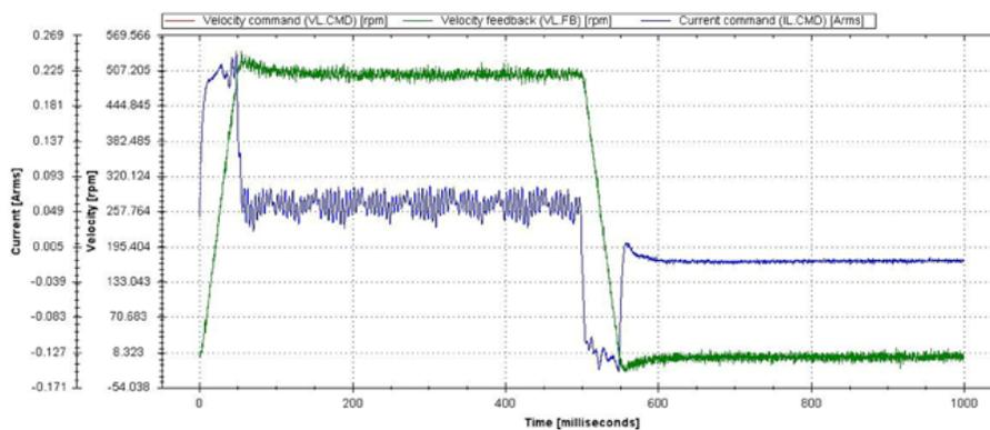
Scope plot showing velocity command and velocity with a velocity closed loop system.
