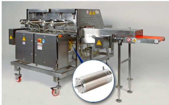
This solution eliminated areas where soil and bacteria can hide — and there's no need to disassemble, clean, sanitize and reassemble prior to each use. It is very easy to clean and sanitize in its place, saving a significant amount of time. **The unenclosed Stainless Steel W series motor takes only 3 minutes to clean versus an enclosed motor that could take up to 20 minutes.** It is also easy to swab the entire machine to verify cleanliness.
