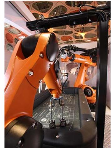
The compact robots with Kollmorgen servo motor drive are especially good at handling tasks, particularly pick-and-place operations.
