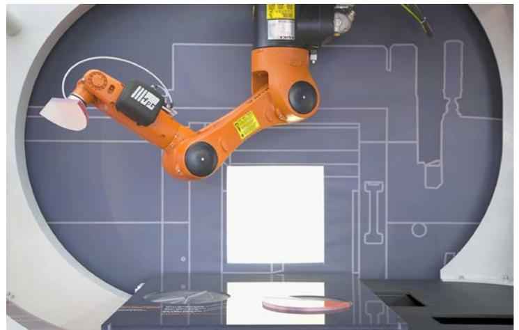
*Thanks to special brakes on all axes, the compact Kuka robots deliver outstanding performance in every position. Kollmorgen found a good solution in cooperation with its brake supplier.*
