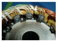
Hall-effect devices are digital On/Off sensors used to sense the presence of magnetic fields. Hall-effect devices come in stand-alone packages that are mounted within the servomotor housing. In brushless servomotors, these sensors are sometimes embedded in the stator windings and switched by the rotor magnets. These devices report the shaft's position, which can also be converted to speed or acceleration data.
