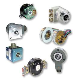
Encoder makers offer several types of discs that generate as many as two million counts per revolution and algorithms that decode them for extremely high resolution positioning. Encoders typically come with multiple channels, such as A and B, and their compliments to wash out any noise pulses that might contaminate the signal. Other signals and their compliments provide a reference position marker for homing and commutation.
